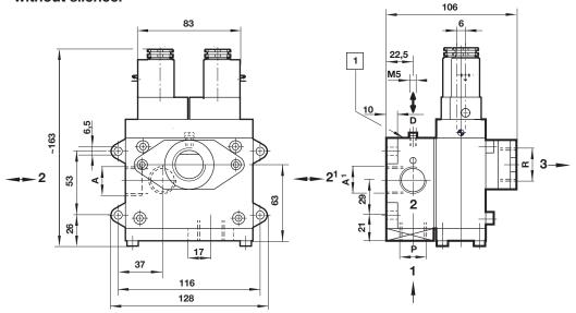
1 Flange surface for pressure switch and failure indicator unit
