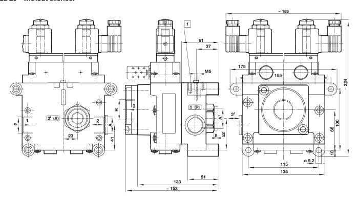
1 Flange surface for pressure switch and failure indicator unit
