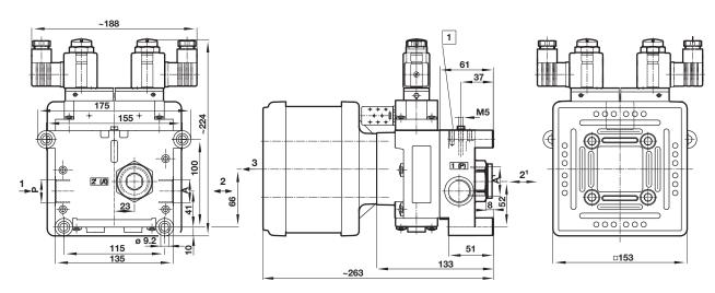
1 Flange surface for pressure switch and failure indicator
